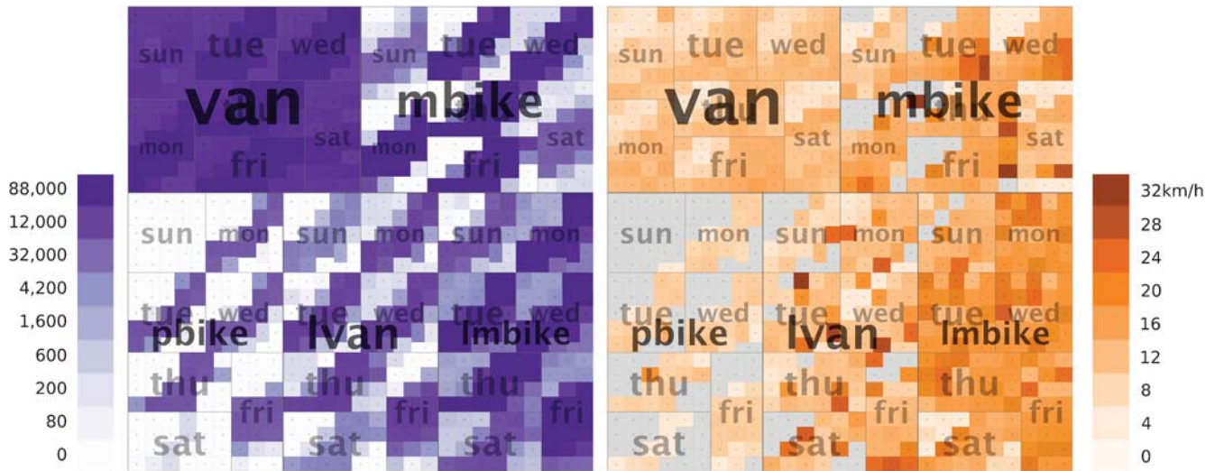
Figure 3 Squarified treemaps showing the same data as in Figure 2 but with fixed leaf sizes and temporal ordering (midnight is at the top left), coloured by traffic volume (purple; logarithmic scale; numbers of points) and average speed (orange; grey where there are no vehicles; km/h). Traffic volume is coloured using ColorBrewer 'Purples' 22 throughout this paper.
